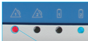
Visual Alarm On
